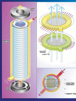
The present invention relates to equipment and process for closed loop circulation cooling tower. This invention uses hydrophobic microporous hollow fiber membrane which is permeable to gas but not permeable to water. Temperature reduction is facilitated by introducing air into liquid phase, which will subsequently be separated in hydro-cyclone unit.
