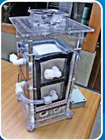
Closed circulation system avoids cooling water contamination by particles and microorganisms from the air, as often occurs when using conventional cooling tower. Thus, fouling on heat exchanger wall can also be prevented since membrane is used as contacting device.
